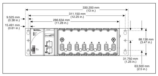
Figure 6. Dimensions of NI 9144 Chassis with Panel Mount Accessory Installed
